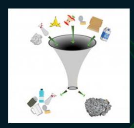
The Fiberight process recovers discreet cellulosic material from inconsistent streams and converts it to products like lactic acid
